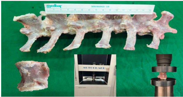
Figure 2. Appearance of the isolated vertebra and the treated vertebra, along with the biomechanical force-impact testing procedure performed using the Shimadzu Autograph AG-IS 100 machine.
